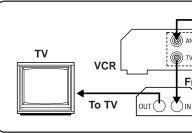
With this connection, you can view one scrambled cable channel while recording another unscrambled channel.
